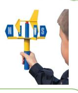
Wind vane — to measure wind direction. They point in the direction in which the wind is blowing from. You may also need a compass to identify the direction.
