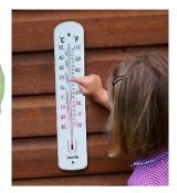
Thermometer — to measure temperature, usually in °C. They will usually record a positive reading, but can fall to minus figures (below freezing).
